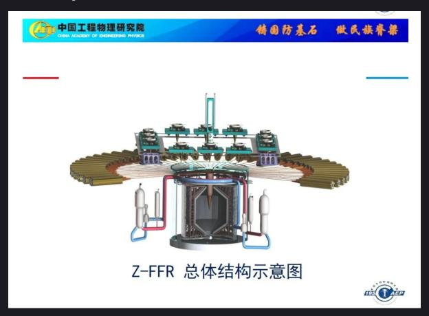
A diagram of the overall structure of China's planned Z Fusion Fission Reactor. Photo: China Academy of Engineering Physics
